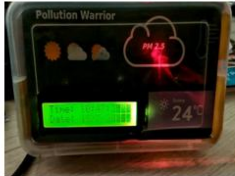
Fig4: Air Quality monitoring device
